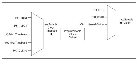
Figure 5-3. Analog Output Timing Options
